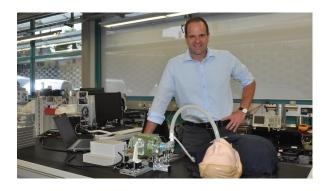
Thermoplan Lung ventilator – based on 80% coffee machine components (mass production of 800 per week at ¼ cost of an original ventilator
