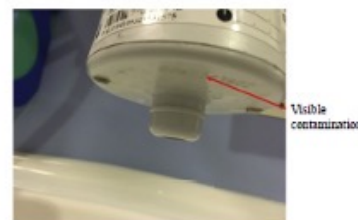
Figure 1. Pall-Aquasafe end filter with visible contamination which yielded multidrug-resistant Pseudomonas aeruginosa .
