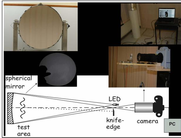
Visualisation of exhaled airflows in real-time from human volunteers using schlieren/shadowgraph mirror-camera set-up – across a 1 m distance (= mirror diameter)
