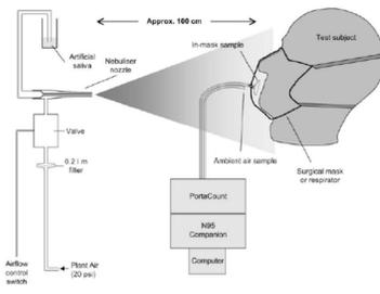
Figure 2.1. Schematic diagram of the inert aerosol test arrangement
