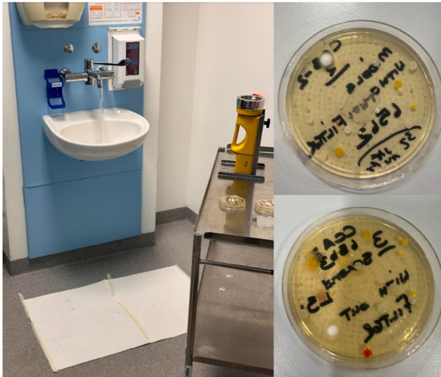
Figure 1. Left: air sampler setup and use with the tap running. Right: examples of the tryptic soy agar plates and micro-c obtained.
